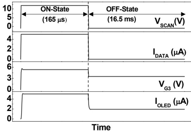
Figure 6. Operation waveforms of the current-scaling current mirror pixel circuit simulated by HSPICE.
