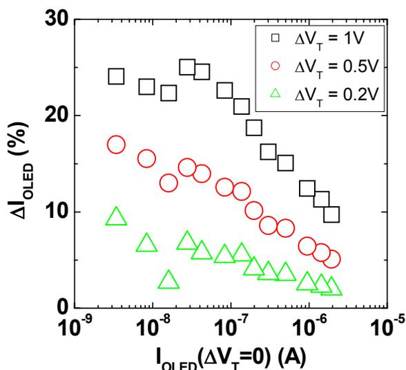
Figure 18.  $\Delta I_{OLED}$  as a function of  $I_{OLED}$  of the 4-TFT current-scaling current-mirror pixel circuit for several levels of  $\Delta V_T$ .
