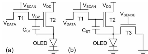
Figure 3. Schematic diagram of the (a) 2-TFT voltage-programmed pixel circuit and (b) the same circuit with an additional TFT (T3).
