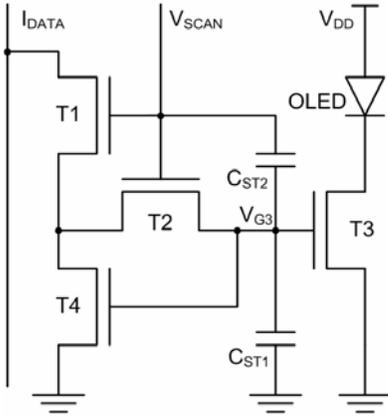
Figure 5. Schematic diagram of the 4-TFT current-scaling current mirror pixel circuit.
