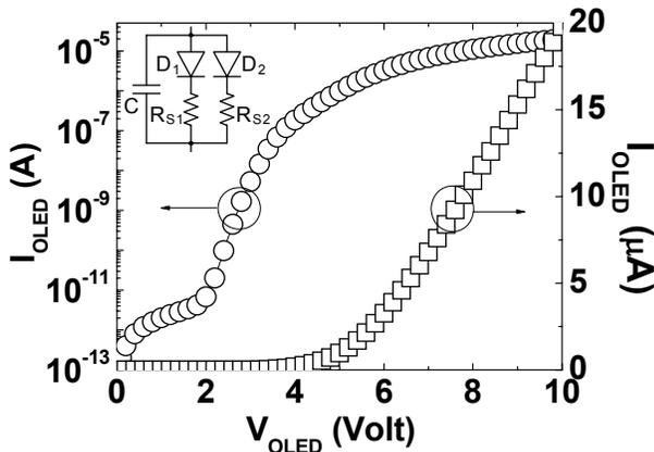
Figure 2. Simulated OLED I-V characteristics
