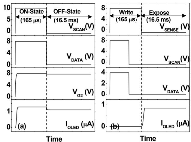
Figure 4. Operation waveforms of the pixel circuits in Fig. 3(a), and (b), respectively, simulated by HSPICE.
