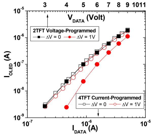
Figure 7. I<sub>OLED</sub> as a function of V<sub>DATA</sub> of the 2-TFT voltage-programmed pixel circuit (solid symbols), and I<sub>DATA</sub> of the 4-TFT current-scaling current-mirror pixel circuit (hollow symbols).
