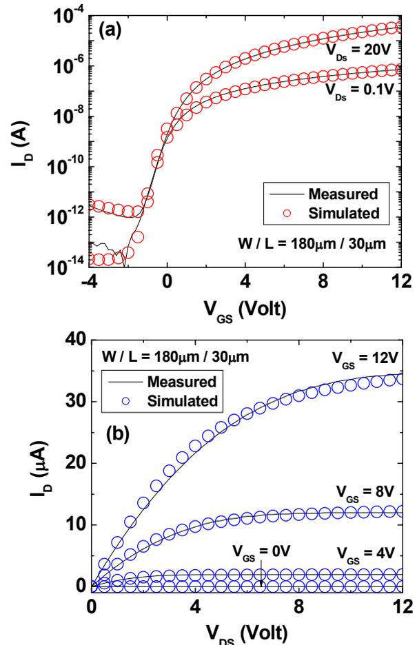
Figure 1. Measured and simulated (by HSPICE) a-InGaZnO TFT (a) transfer characteristics and (b) output characteristics.
